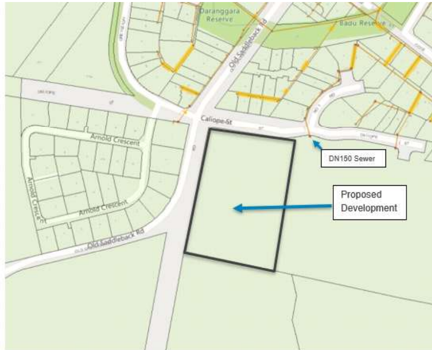
Figure 3 Proposed Development and surrounding sewer mains
